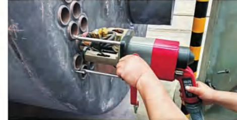
△自动管板焊 Automatic Tube-To-Sheet Welding
