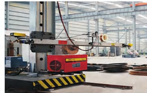
△埋弧自动焊 Automatic Submerged Arc Welding
