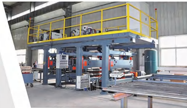
△膜式壁生产线 Membrane Wall Production Line
