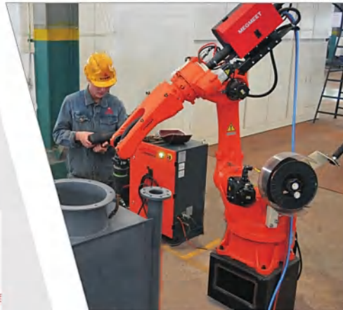
△机器人焊接 Robot Welding
