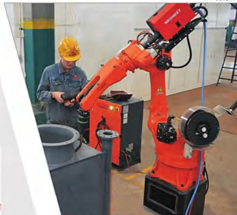
△机器人焊接 Robot Welding
