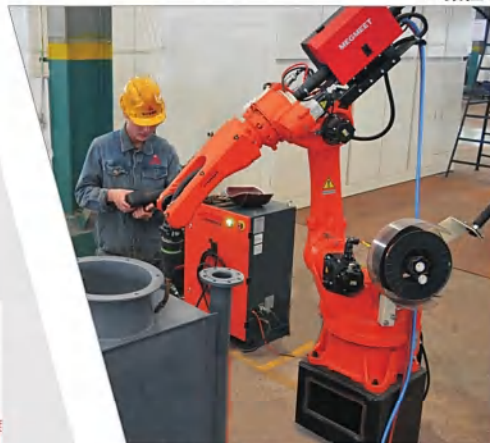
△机器人焊接 Robot Welding
