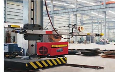
△埋弧自动焊 Automatic Submerged Arc Welding
