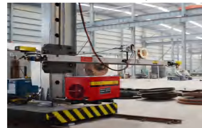
△埋弧自动焊 Automatic Submerged Arc Welding
