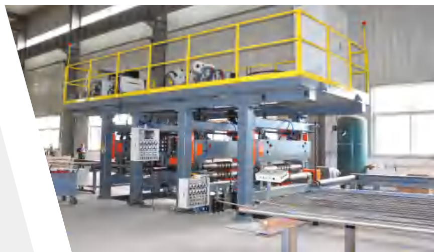
△膜式壁生产线 Membrane Wall Production Line
