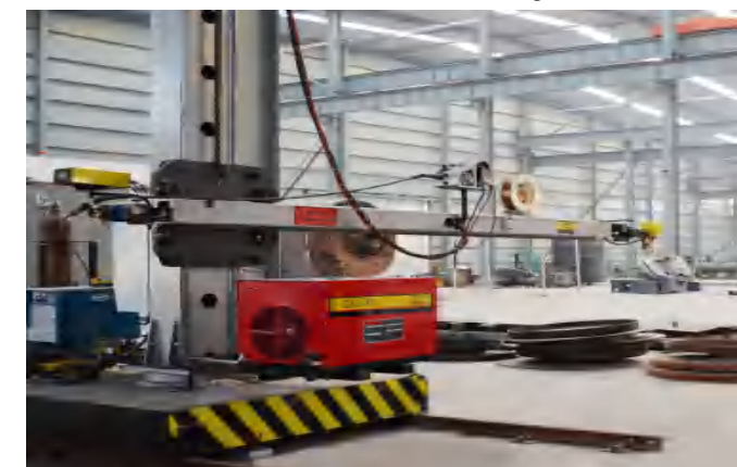
△埋弧自动焊 Automatic Submerged Arc Welding
