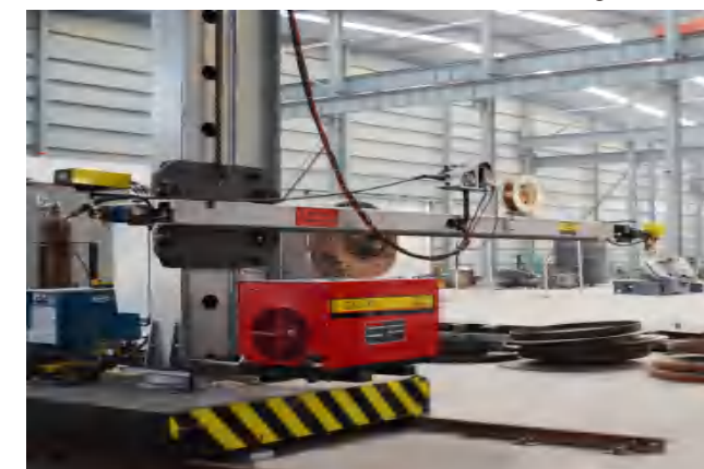
△埋弧自动焊 Automatic Submerged Arc Welding
