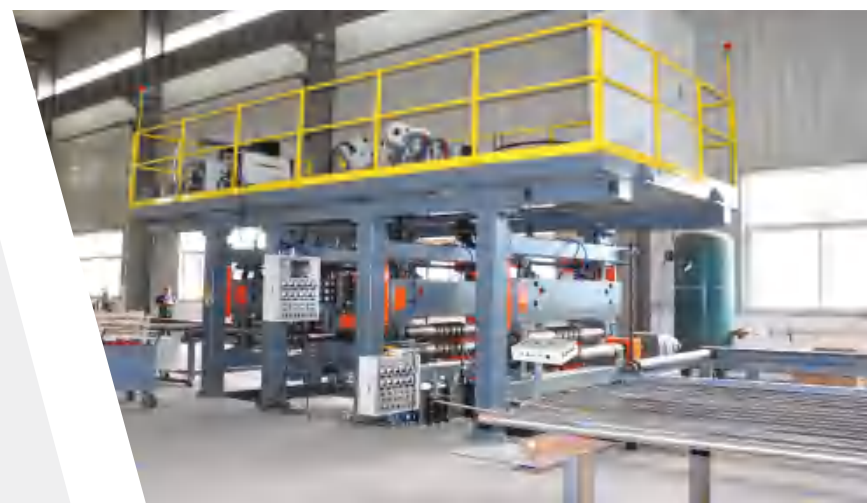
△膜式壁生产线 Membrane Wall Production Line
