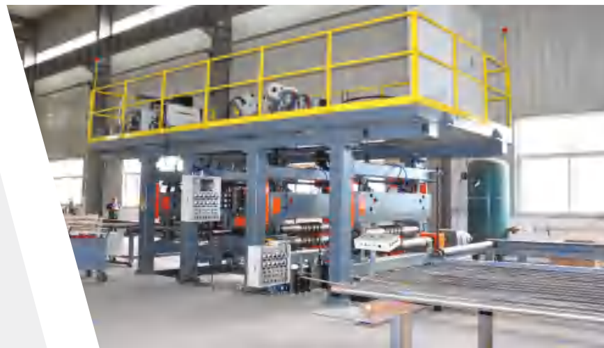
△膜式壁生产线 Membrane Wall Production Line
