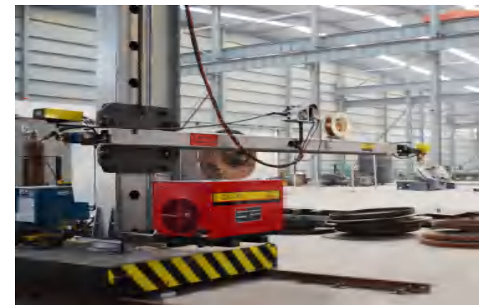
△埋弧自动焊 Automatic Submerged Arc Welding
