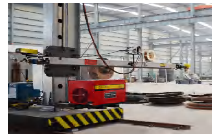
△埋弧自动焊 Automatic Submerged Arc Welding
