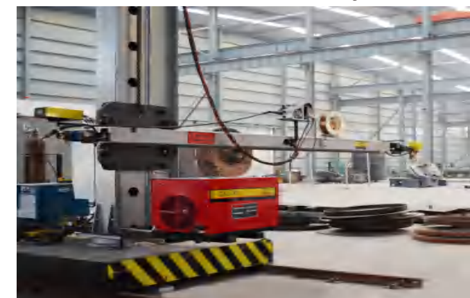
△埋弧自动焊 Automatic Submerged Arc Welding
